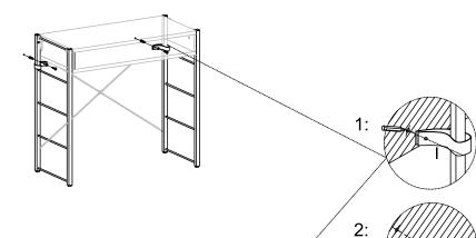
To prevent toppling, wall straps must be positioned below the top rung of each ladder. Ensure the strap is pulled tight before fixing to your wall.
