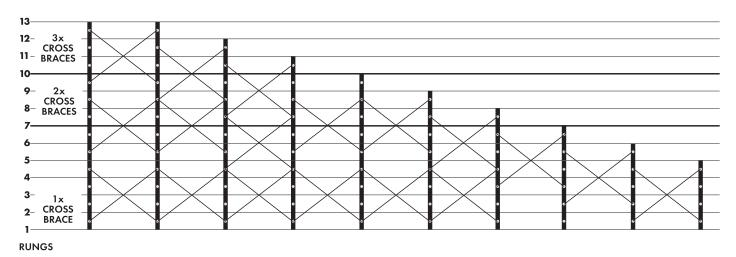
Where possible, we recommend positioning Cross Braces across the joins of the Ladder Bases and Extensions for added stability.
